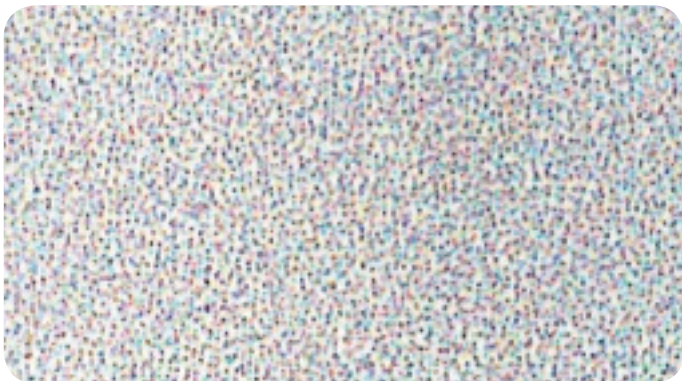
Low level magnification of flat tint on AccurioJet KM-1 showing no lines and artefacts and colour consistency
