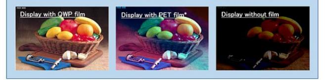
The image of the "Display with PET film" is an example of how an image can appear when PET (polyethylene terephthalate) film is applied on a display in place of QWP film.
